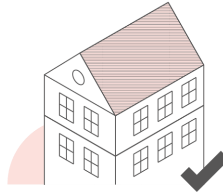
Pitched roof whose entire area is made of PV installation in a built-up area where the existing roof coverings are of non-traditional style and colours with no visual exposure from public and semi-public spaces.
