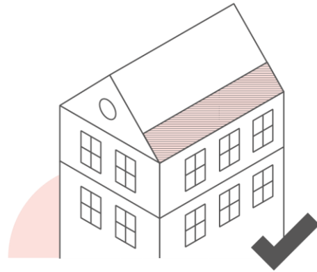
Pitched roof with a later addition of an embedded PV installation (e.g. solar roof tiles) neatly arranged, in colour and size not contrasting with the traditional roof covering in the area and not visually exposed from a public and semi-public spaces.
